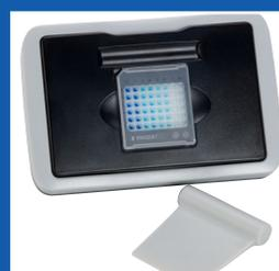
Load samples in plate using the convenient Eco 48 sample loading dock.
