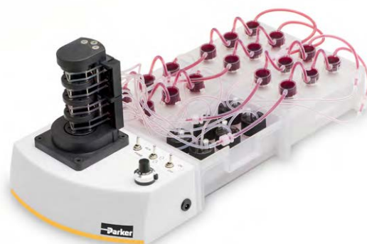
QV900 with integrated Parker Polyflex peristaltic pump
