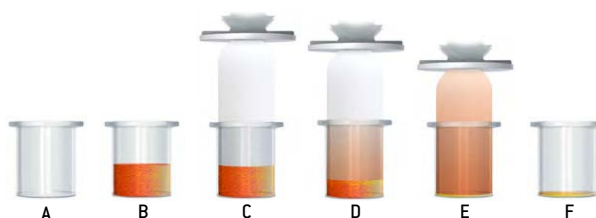
RAFT™ Sequence (A) Empty well or insert, (B) Cell and collagen mix forms hydrogel at 37°C, (C) Absorber contacts the hydrogel, (D) Liquid starts to be absorbed, (E) Process concentrates cells and collagen, (F) In less than 1 hour culture formation complete.
